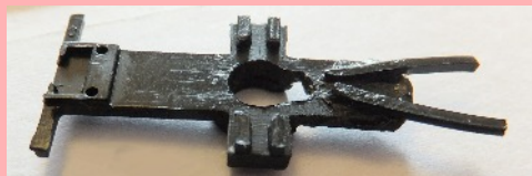
Bolster with auto-close up/open-out coupling mechanism operating strips attached
