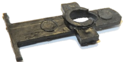
Ultima bolster with coupling fitting removed, fixing pin head glued in place and cut/drilled to clear pivot and lug
