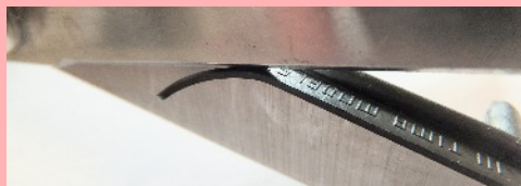
Cutting strip from top tab of sprue
